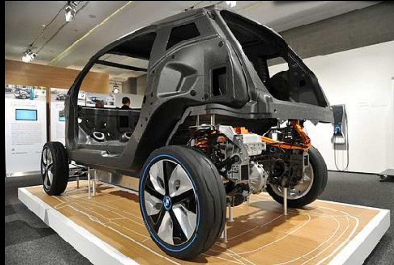
BMW MY2013's ~120–150-kg carbon-fiber-composite passenger cell; m_c 1,250 kg
